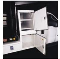
**Reading's REV-PAC compartments** mount neatly between the body and cab for extra weathertight storage space.
