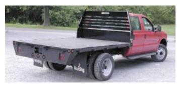
**Reading's Redi-Dek®** comes standard with slotted bulkhead, a rear apron, and tie-down rails
