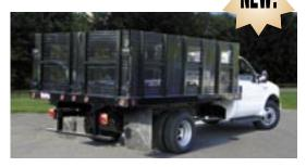
**Redi Racks** provide the ability to haul loose bulk loads without the weight of solid sides (body shown also equipped with an optional REV-PAC)
